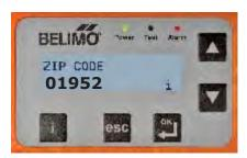
MAKE SURE ZIP CODE IS NOT FLASHING. IF IT IS, PRESS OK ONE MORE TIME TO MAKE NUMBERS SOLID. NOW PRESS ESC ONCE
