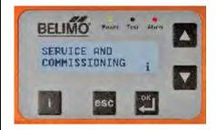
PRESS DN TILL AT THIS SCREEN AND PRESS "OK"
