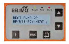
USING "UP" AND "DN" ARROWS SET EITHER [B],[O], OR [W1] PRESS "OK"
