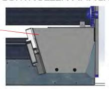
2 SCREWS LOCATED HERE FOR BRACKET REMOVAL
