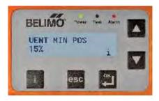
PRESS THE DOWN ARROW UNTIL YOU GET TO THE VENT MIN POS MENU. NOW PRESS OK AND THE % WILL BEGING TO FLASH. USE UP ARROW AND SET YOUR MIN. O/A % THEN PRESS OK
