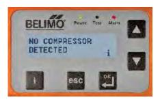
PRESS "DN" ONCE TO "NO COMPRESSOR DETECTED" SCREEN. PRESS "OK"
