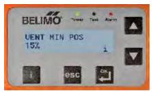
OPERATION: OUTSIDE AIR DAMPER WILL MODULATE BETWEEN DCV MIN (MINIMUM) AND VENT MIN(MAXIMUM) TO KEEP SPACE CO2 LEVELS BELOW SETPOINT
