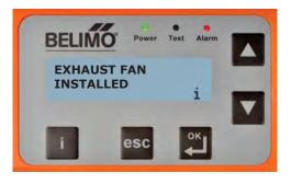
IN THE SETTINGS MENU SCROLL DOWN TO THE DEVICES 1 MENU AND PRESS OK. NEXT SCROLL DOWN TO EXHAUST FAN AND PRESS OK. NOW SET EXHAUST FAN TO INSTALLED USING DN ARROW. THEN PRESS OK. LASTLY PRESS ESC TO GET BACK TO SETTINGS.
