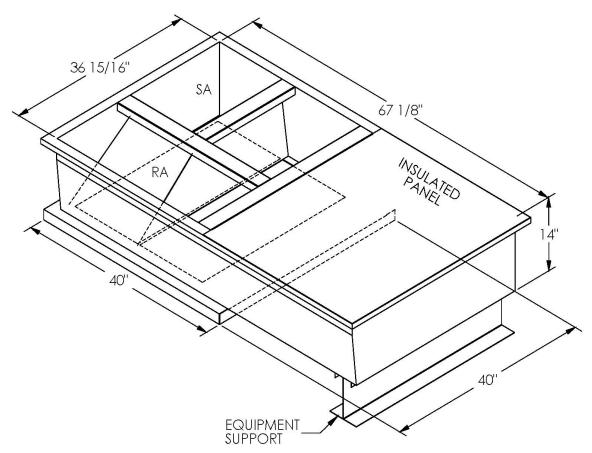
ONE PIECE WELDED CONSTRUCTION
