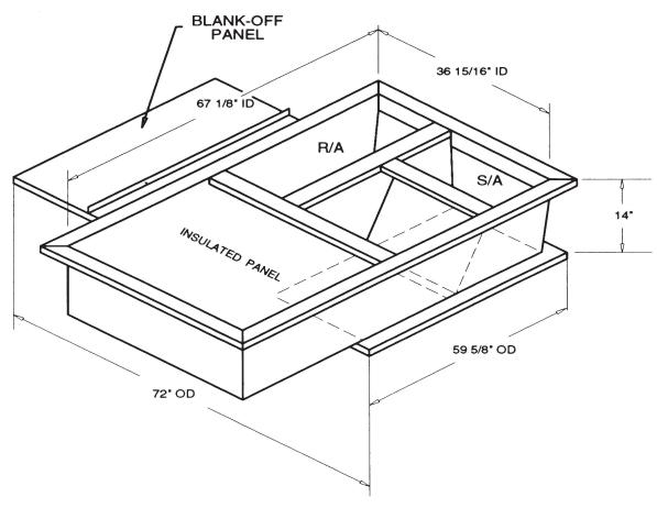
ONE PIECE WELDED CONSTRUCTION
