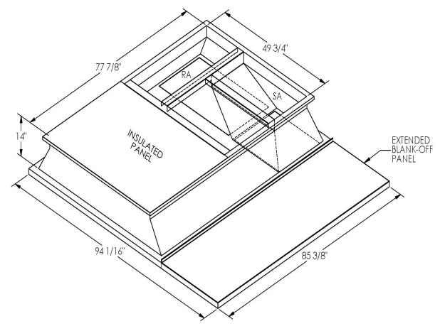
ONE PIECE WELDED CONSTRUCTION
