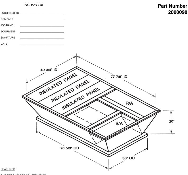
ONE PIECE WELDED CONSTRUCTION
