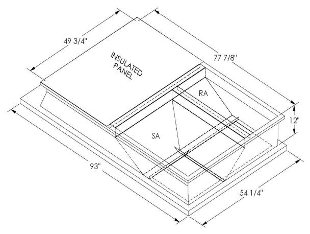
ONE PIECE WELDED CONSTRUCTION
