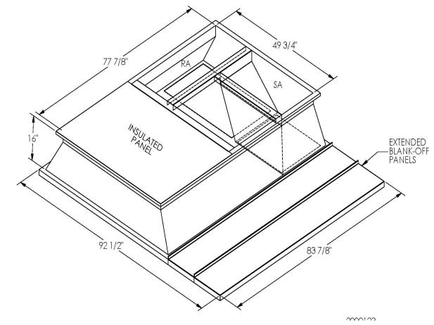
ONE PIECE WELDED CONSTRUCTION
