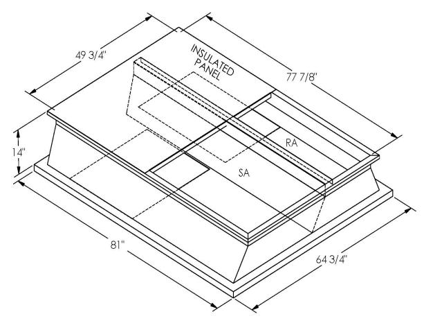
ONE PIECE WELDED CONSTRUCTION
