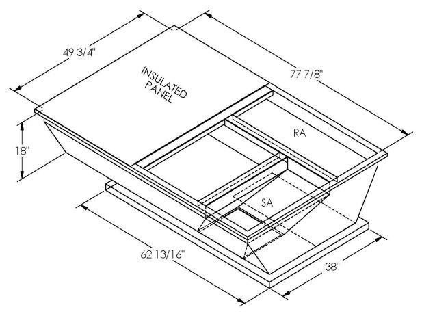
ONE PIECE WELDED CONSTRUCTION
