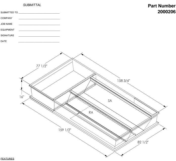
ONE PIECE WELDED CONSTRUCTION
