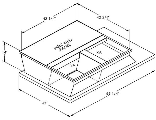
ONE PIECE WELDED CONSTRUCTION
