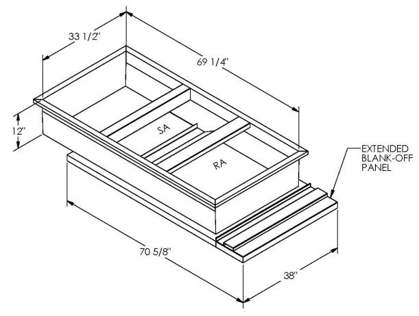
ONE PIECE WELDED CONSTRUCTION
