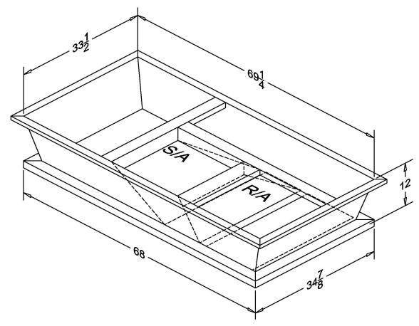
ONE PIECE WELDED CONSTRUCTION
