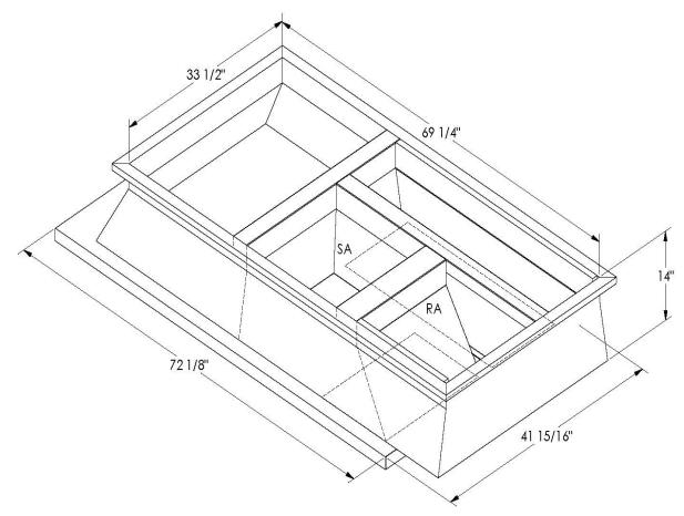
ONE PIECE WELDED CONSTRUCTION
