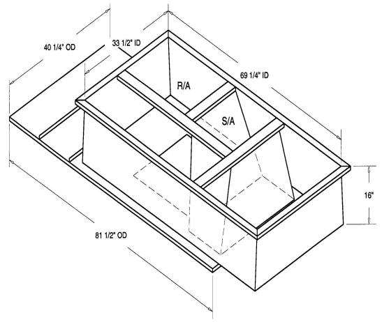
ONE PIECE WELDED CONSTRUCTION
