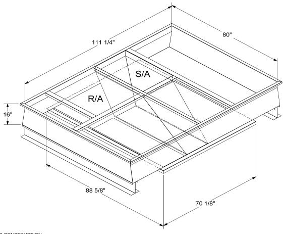
ONE PIECE WELDED CONSTRUCTION
