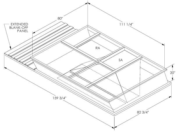
ONE PIECE WELDED CONSTRUCTION
