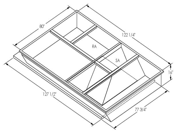
ONE PIECE WELDED CONSTRUCTION
