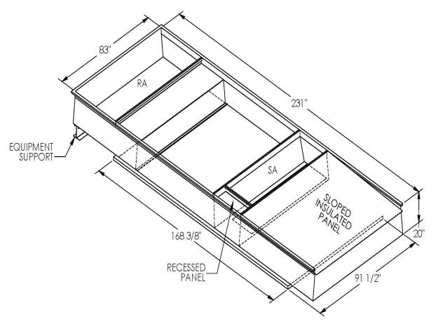
ONE PIECE WELDED CONSTRUCTION
