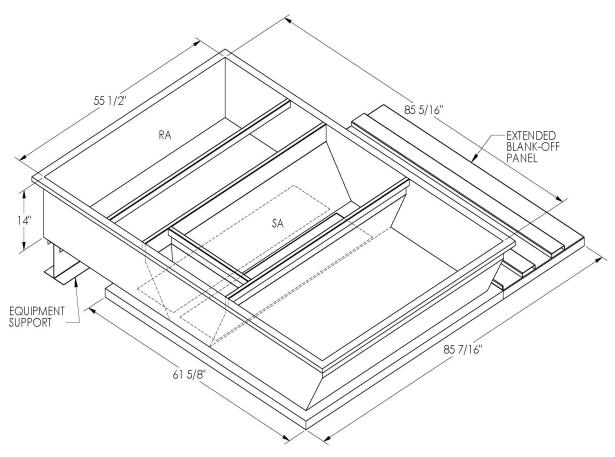
ONE PIECE WELDED CONSTRUCTION
