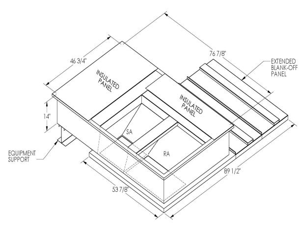
ONE PIECE WELDED CONSTRUCTION
