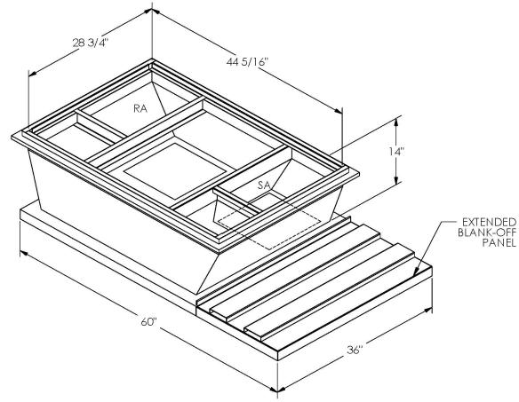
ONE PIECE WELDED CONSTRUCTION
