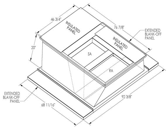
ONE PIECE WELDED CONSTRUCTION
