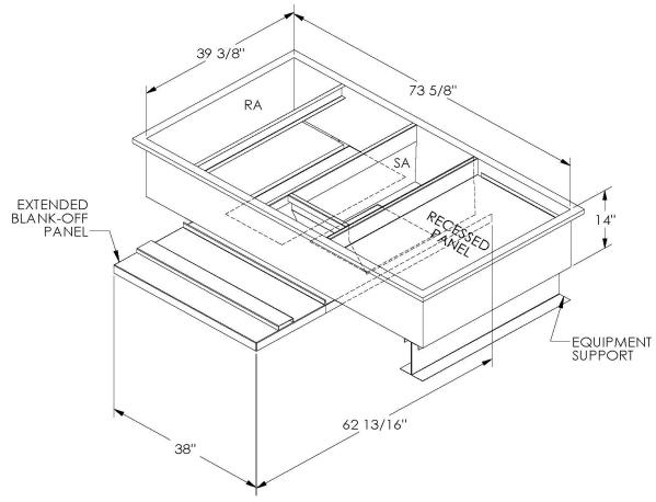
ONE PIECE WELDED CONSTRUCTION
