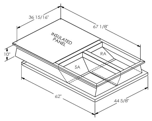
ONE PIECE WELDED CONSTRUCTION
