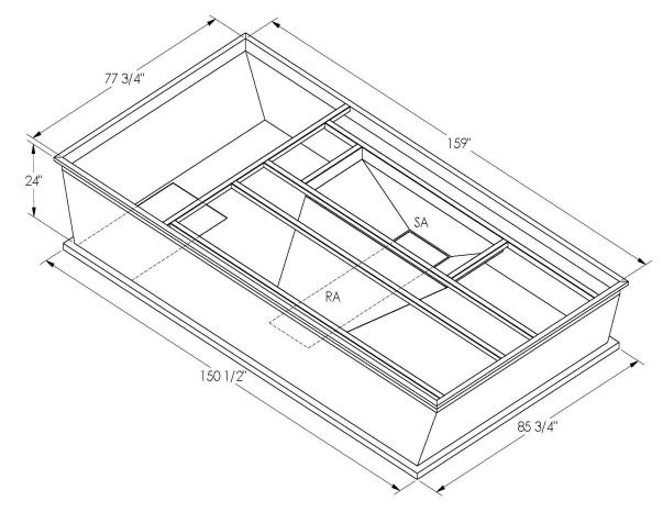
ONE PIECE WELDED CONSTRUCTION
