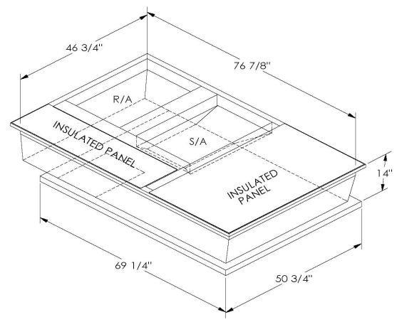
ONE PIECE WELDED CONSTRUCTION
