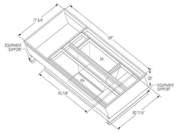
ONE PIECE WELDED CONSTRUCTION
