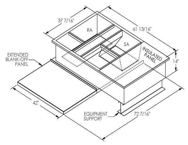
ONE PIECE WELDED CONSTRUCTION
