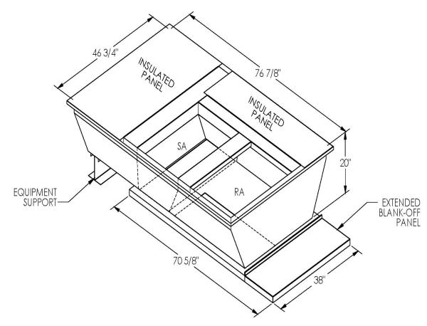
ONE PIECE WELDED CONSTRUCTION
