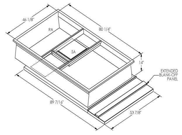
ONE PIECE WELDED CONSTRUCTION
