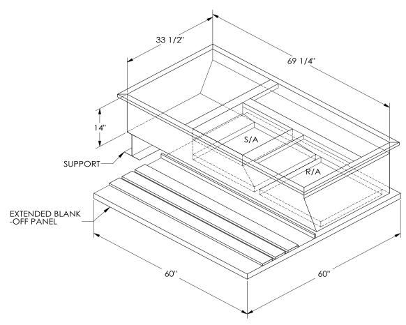
ONE PIECE WELDED CONSTRUCTION
