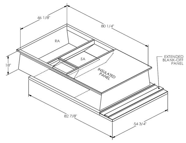
ONE PIECE WELDED CONSTRUCTION
