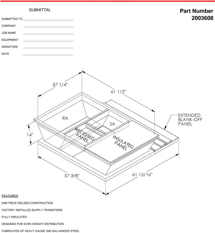
ALL WELDS SPRAYED WITH GALVANIZING COMPOUND
