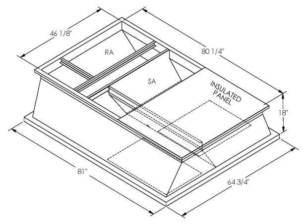
ONE PIECE WELDED CONSTRUCTION
