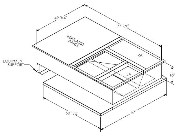
ONE PIECE WELDED CONSTRUCTION
