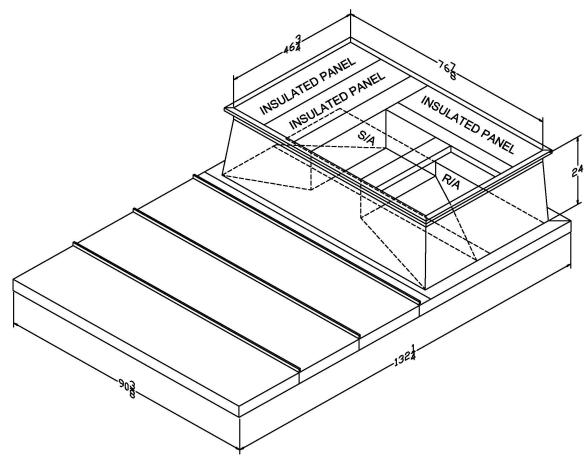
ONE PIECE WELDED CONSTRUCTION
