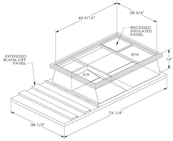
ONE PIECE WELDED CONSTRUCTION
