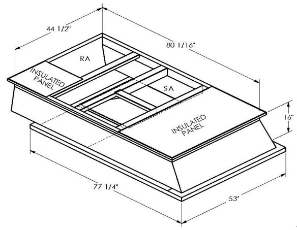
ONE PIECE WELDED CONSTRUCTION
