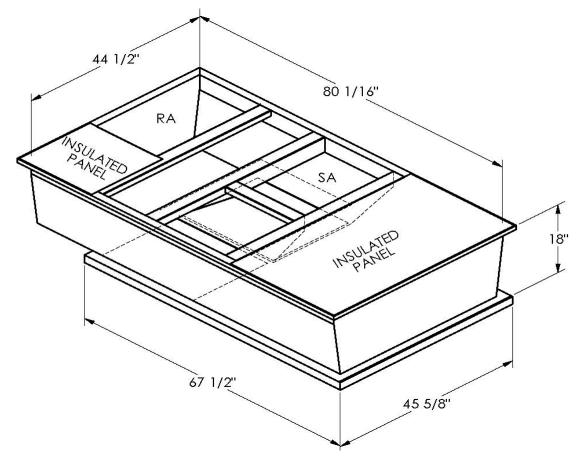
ONE PIECE WELDED CONSTRUCTION
