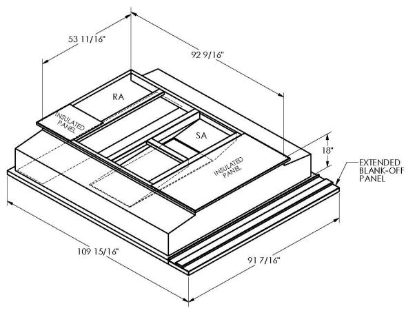
ONE PIECE WELDED CONSTRUCTION
