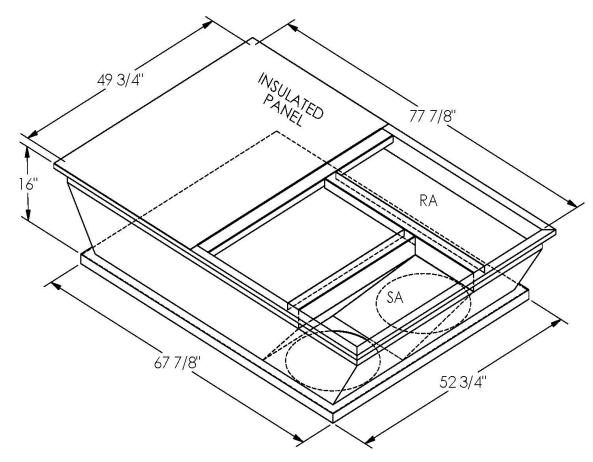
ONE PIECE WELDED CONSTRUCTION
