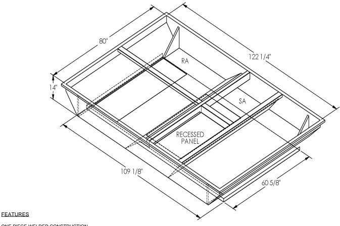
ONE PIECE WELDED CONSTRUCTION
