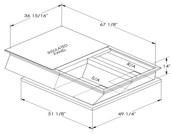
ONE PIECE WELDED CONSTRUCTION
