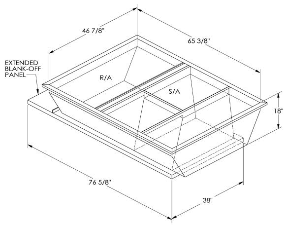
ONE PIECE WELDED CONSTRUCTION
