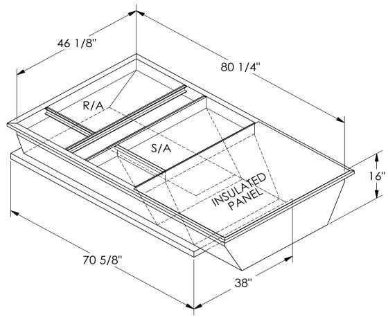
ONE PIECE WELDED CONSTRUCTION
