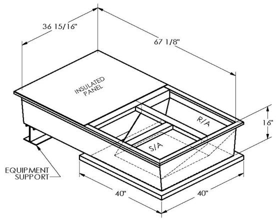
ONE PIECE WELDED CONSTRUCTION
