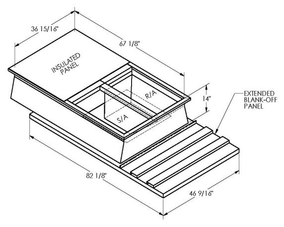
ONE PIECE WELDED CONSTRUCTION
