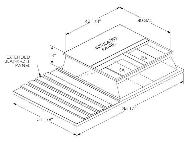
ONE PIECE WELDED CONSTRUCTION
