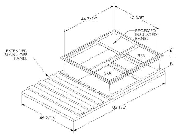
ONE PIECE WELDED CONSTRUCTION
